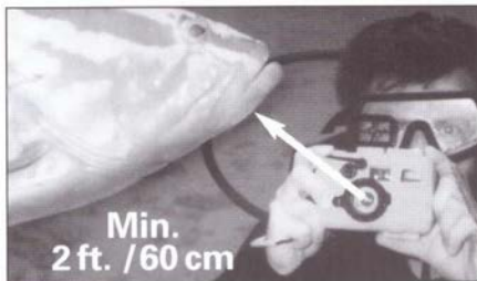
Minimum distance with close-up lens
