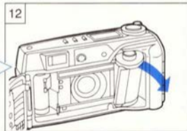
12 Open the back cover to remove the rewind film (p. 23).
