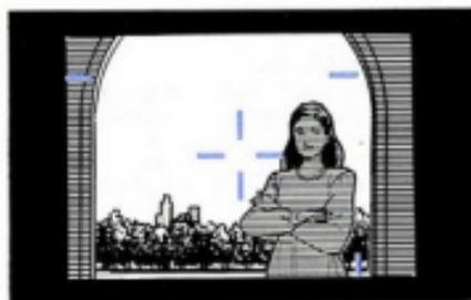
In the case shown on the left, the camera will set the exposure for the background in the normal mode.
