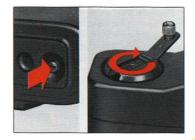
The film is fully rewound when the crank starts turning more freely.
