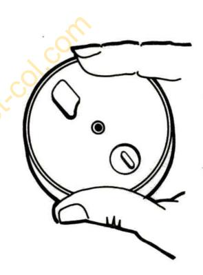
are on top facing you and the gear is on the bottom. Place the Filmdisk in the back compartment of the camera with the gear down. The raised rectangle part of the Filmdisk ™ should be directly below the viewfinder. Close the camera. A slight click when the viewfinder sections come together indicates that the camera is completely closed. Note: the shutter release should be in the "picture taken" position when placing a Filmdisk ™ in the camera. Do not reset.
